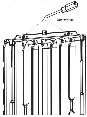
Snap Repeat Left Side (C) into the back position of Repeat Floor (B).
